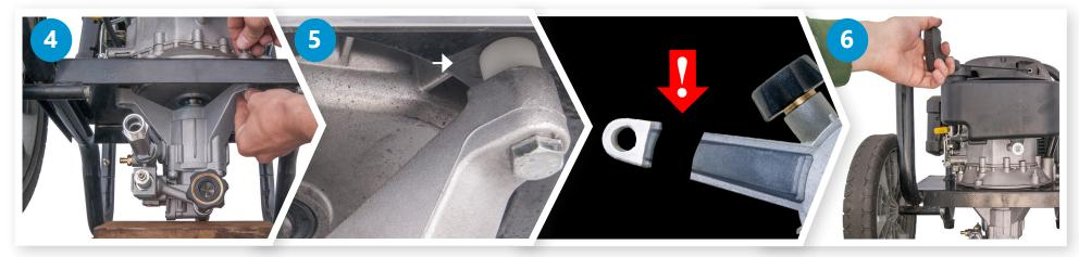
Line up the pump arms with the mounting holes on the frame/engine. Use an object (brick, wood, etc) to support the pump and install nuts and bolts one at a time. **Do not tighten yet.**
