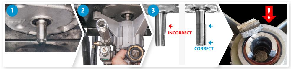
TOOLS NEEDED: 1/2" line wrench, 1/2" socket, rachet, nuts and bolts from old pump, spacers and shaft key (provided).
